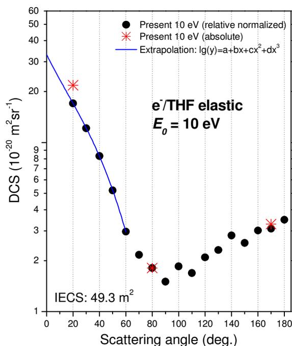
**Figure 2.** Angular dependence of absolute DCS for elastic electron scattering from THF at the incident energy of 10 eV: \*, present absolute measurements obtained by relative-flow method; ●, present relative measurements, normalized at  $20^\circ$  (statistical errors are less than symbol sizes); --, extrapolation of the DCS down to  $0^\circ$ .
