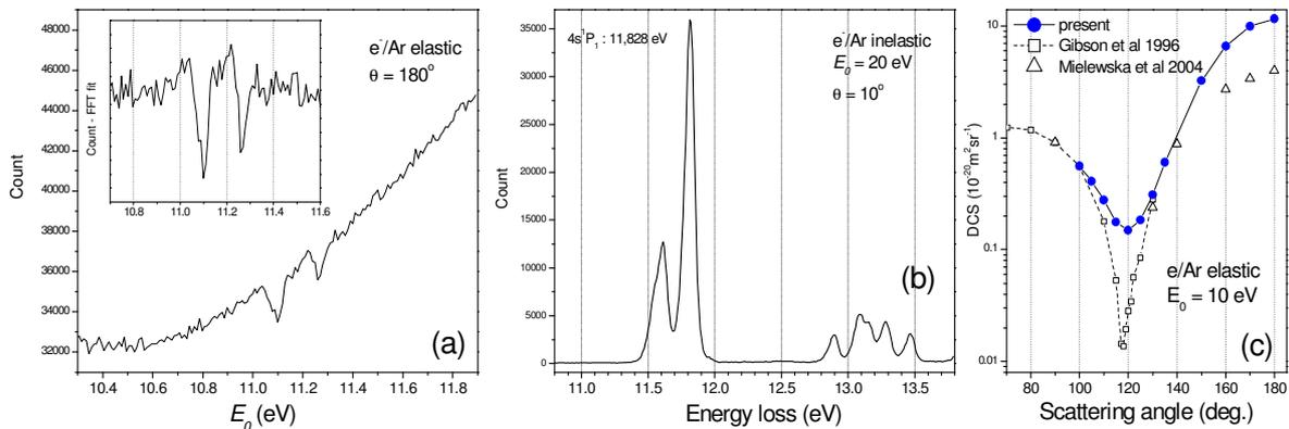
**Figure 1.** Test measurements for Ar: (a) Elastic scattering intensity as a function of incident electron energy ( $E_0$ ). (b) Energy loss spectrum of Ar at the incident energy of 20 eV and scattering angle of  $10^\circ$ . (c) DCS for elastic electron scattering by Ar at 10 eV, in the vicinity of the minimum.
