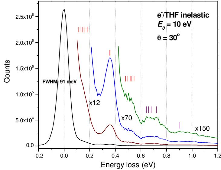
**Figure 3.** Vibrational energy loss spectrum of THF recorded at incident electron energy of 10 eV and at scattering angle of  $30^\circ$ . The marked vibrational levels are either taken from [2] (red bars) or represent present suggested combination losses (purple bars).
