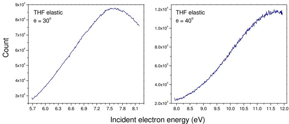
**Figure 4.** Elastic electron-THF scattering intensity as a function of incident electron energy at scattering angles of  $30^\circ$  and  $40^\circ$ .
