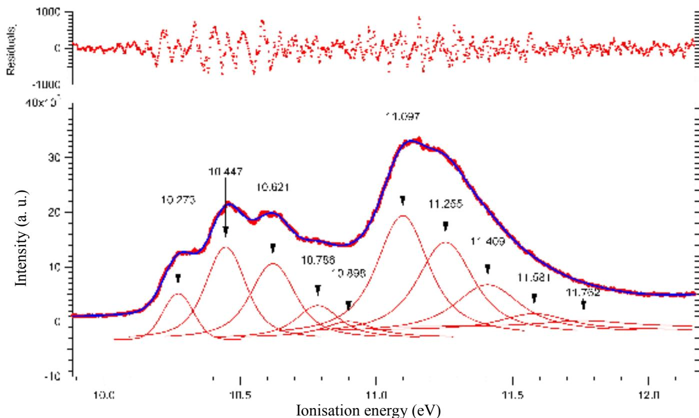
Figure 2 Voigt function fit and ionisation energies assignment for methyl acetate.
