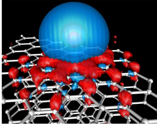
**Figure 2.** Electron density accumulation/depletion isosurfaces of a K adatom on graphite (density difference values  $\pm 0.0005 e/a_0^3$ ). Color key: Red, accumulations; blue, depletion.
