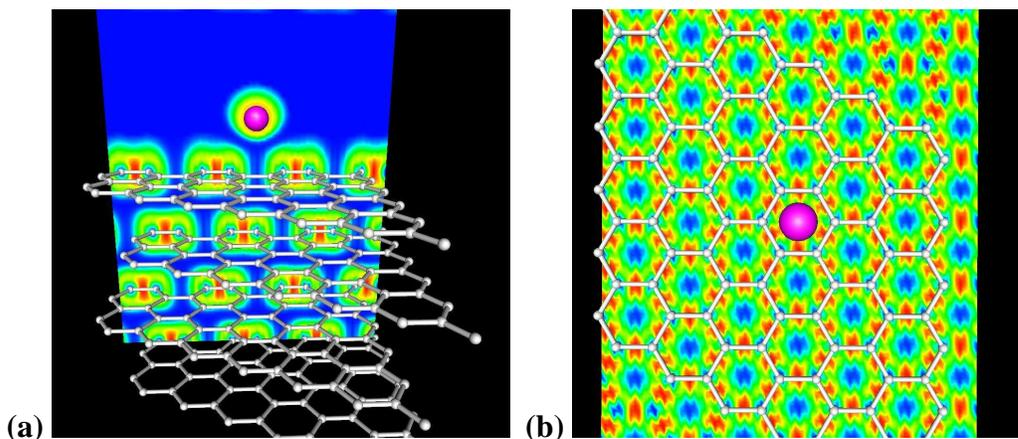
**Figure 4.** Electron localization function (ELF) of K adatom on graphite. Color key: Red, localization (covalent bonding); green, metallic bonding (homogeneous electron density); and blue, no overlap.
