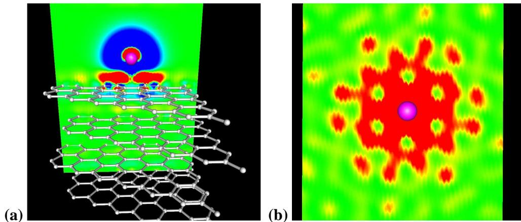
**Figure 3.** Cutplane representations of the charge density redistribution. Color key: Red, accumulations; blue, depletion.
