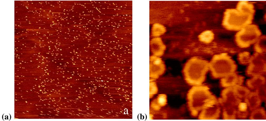
**Figure 1.** STM images of K islands on graphite. (a) Dispersed phase of K adatoms and clusters, and (b) nanoscale K islands and sparsely distributed K adatoms (weak features).
