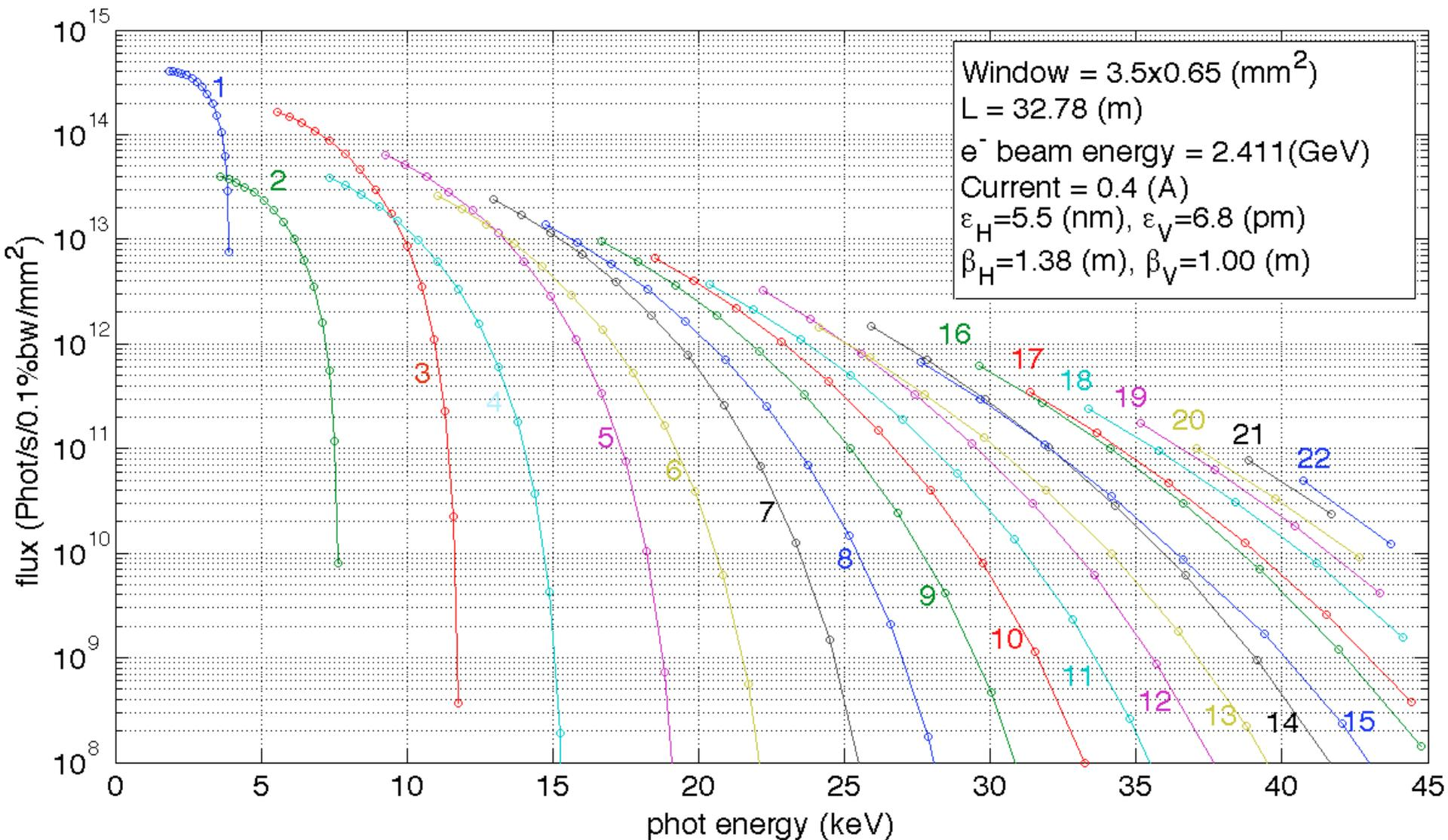
Phase error  $< 2.5^\circ$  RMS for gap 4.6 mm  $\Rightarrow$  50% at  $n = 19$
