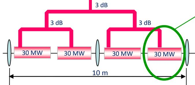
four 2 m long C-band structures, 30 MV/m
