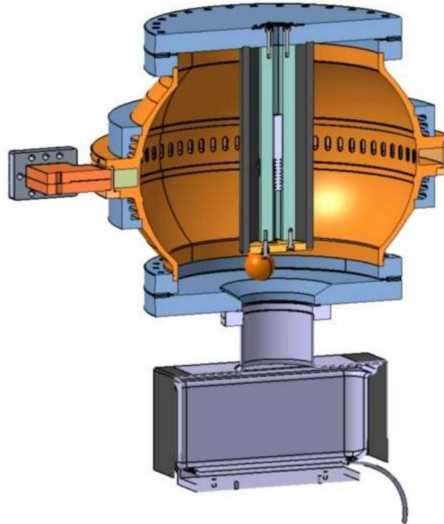
BOC (barrel-open cavity)
