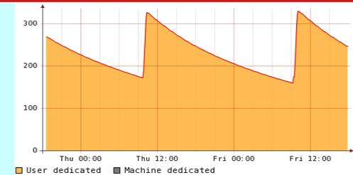
**Decay mode, 2 GeV (340mA) and 2.4 GeV (140) – SRFEL at 1 GeV.**
