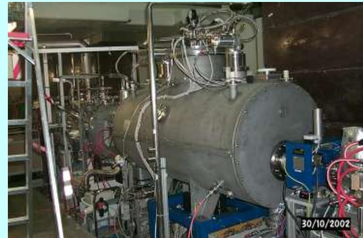
Its consumption as measured in 2004 of 0.6-0.7 l/h would be an additional difficulty with top up operations; however during tests in May 2011 it has been observed: 2 l/h without field and 7 l/h with magnetic field that anyway could not go above 0.9 T
