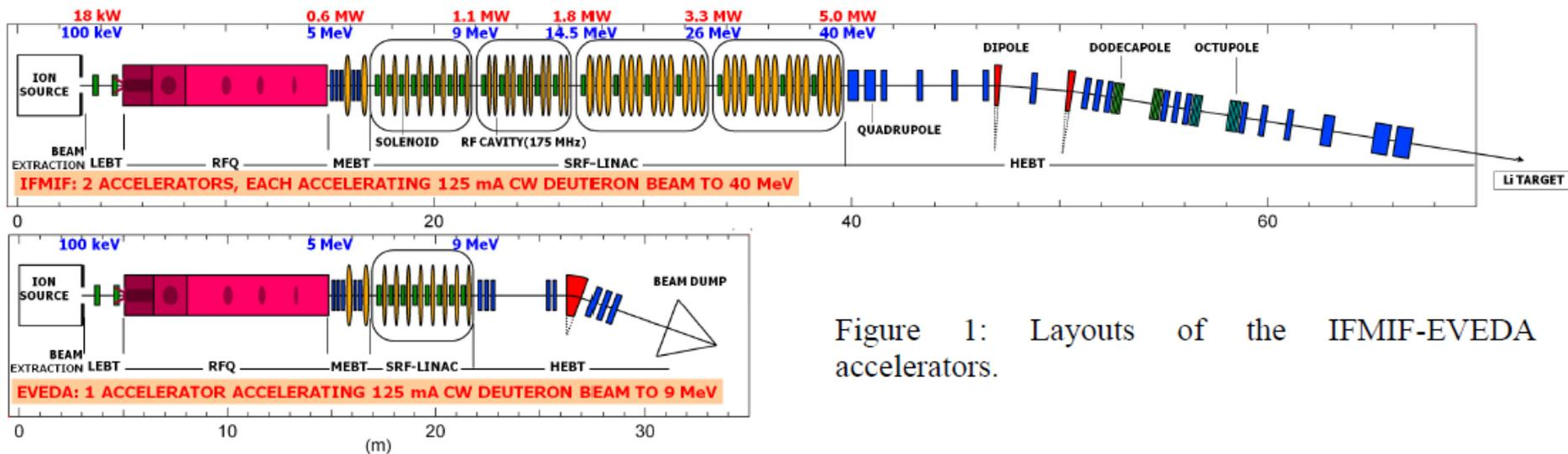
Figure 1: Layouts of the IFMIF-EVEDA accelerators.
