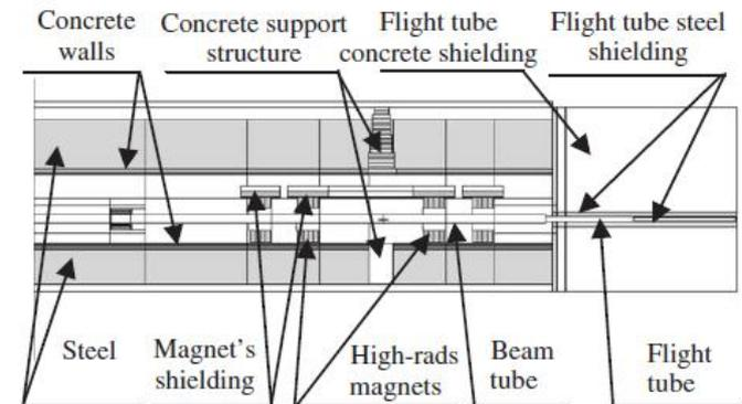
Fig. 5. Model of SNS RTBT T-section and flight tube section, elevation view.
