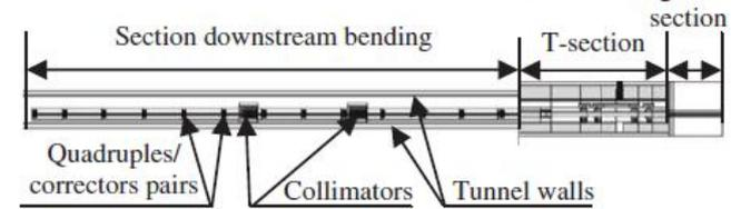
Fig. 4. Model of SNS RTBT portion, elevation view.
