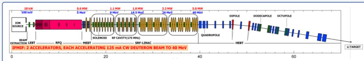
**IFMIF Accelerator:  $2 \times 5 \text{ MW}$**
