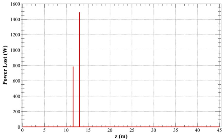
**Total power lost: 2.276 kW – Losses on scrappers**
