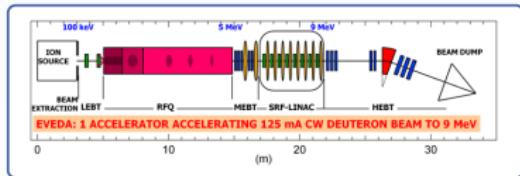
**Linear IFMIF Prototype Accelerator (LIPAc): 1.125 MW**
