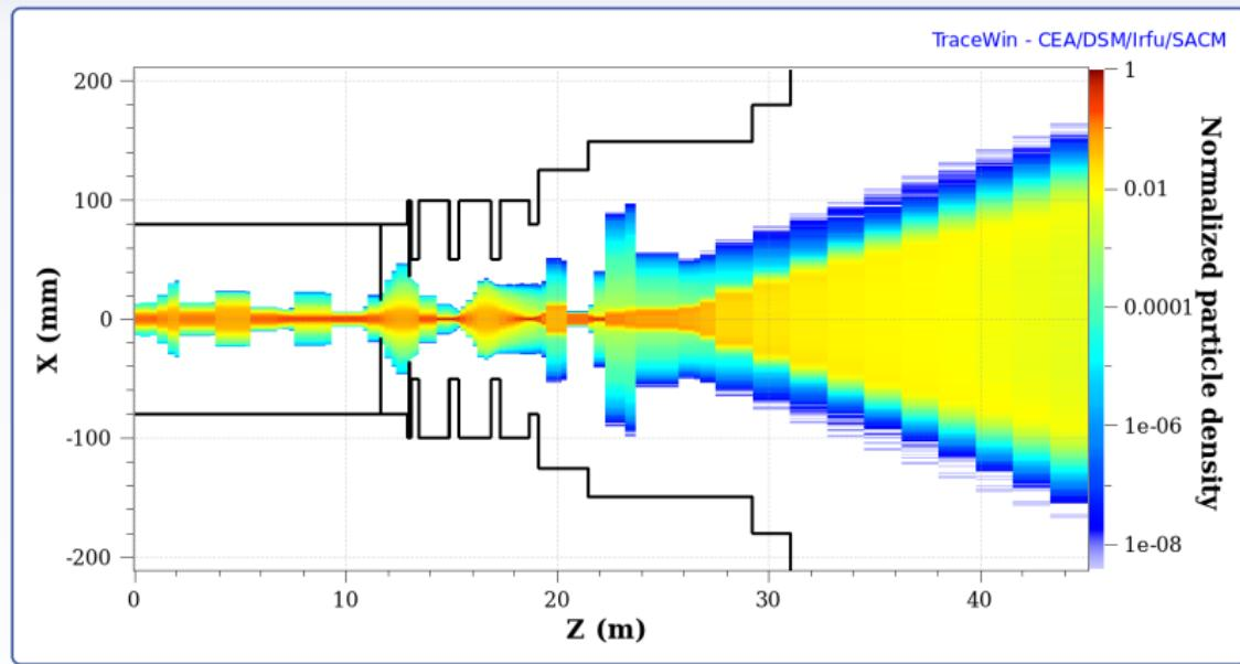
Cumulated Beam (200 runs) Density – X plane – WITH errors
