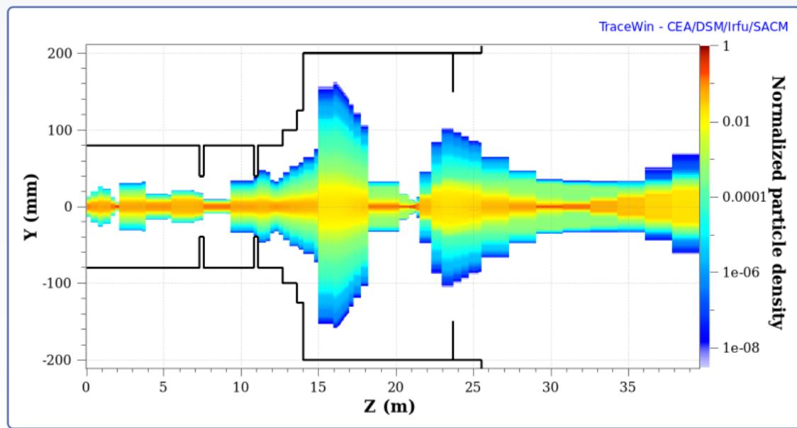
Cumulated (200 runs) Beam Density – Y plane – WITH errors
