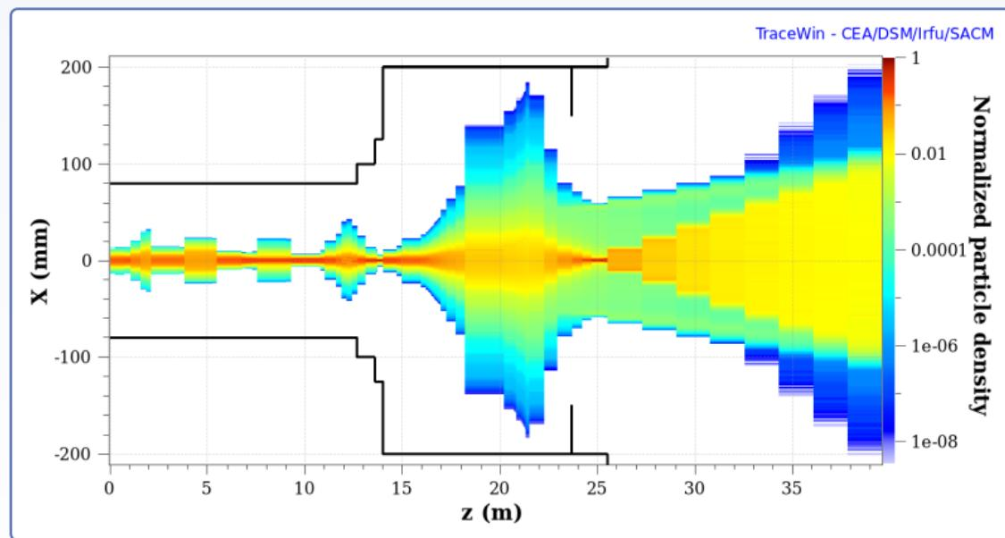
Cumulated (200 runs) Beam Density – X plane – WITH errors
