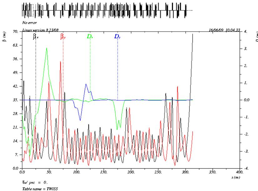
Beam optics for flattening by OCTs
