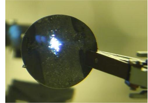
Pin holes at target of SNS
