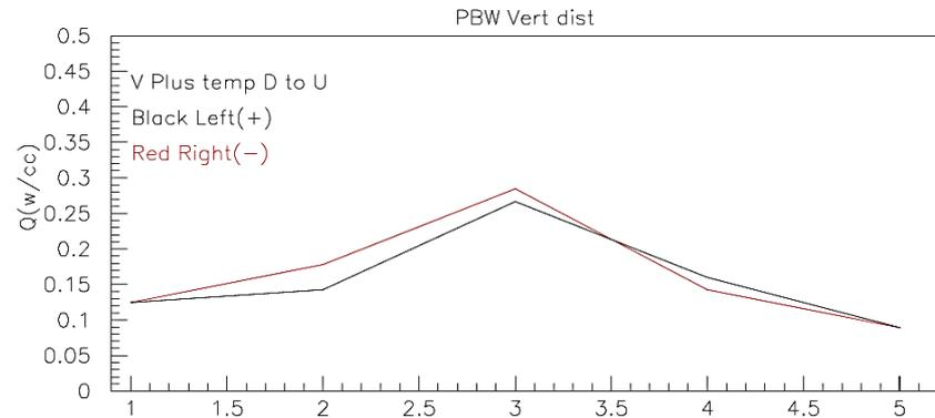
Result of heat deposition at halo monitor
