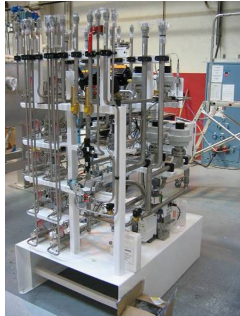
Room temperature valve panel
