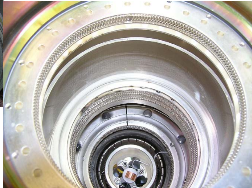
Signs of arcing inside the cavity
