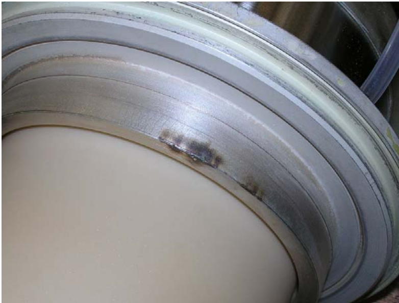
Sign of arcing on the IOTs
