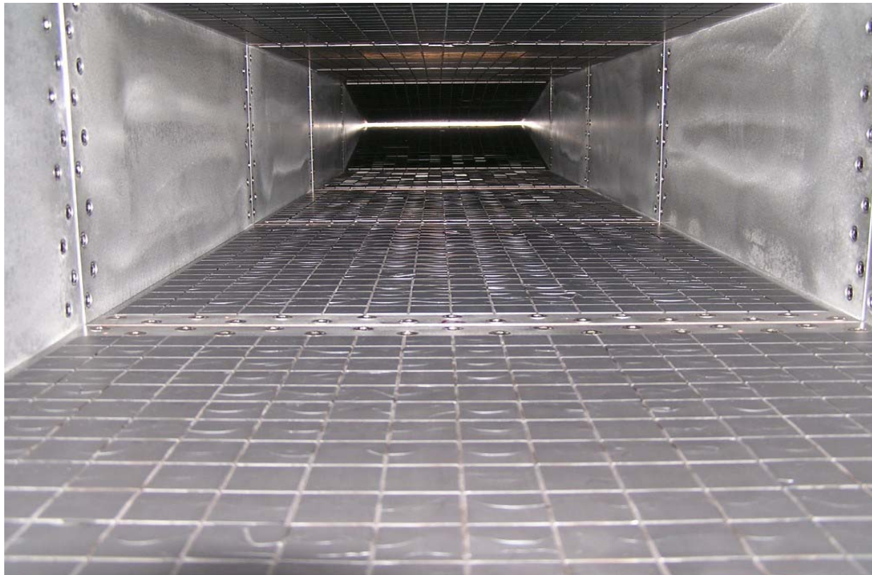
Inside view of ferrite load
