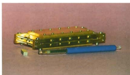
The Micropole Undulator prototype with 4 stacked magnets to the left.
